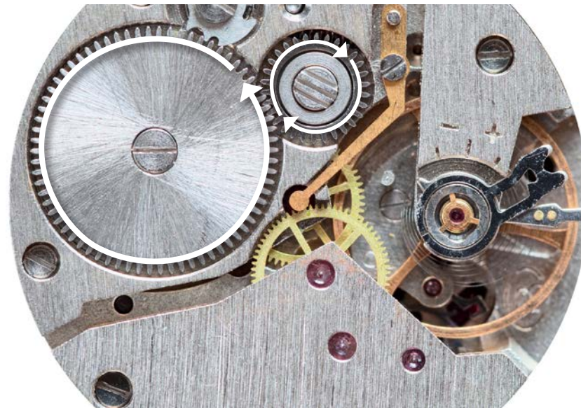
For every time the large gear turns, the small gear turns more than once. The large gear has more force, while the small gear moves faster.
